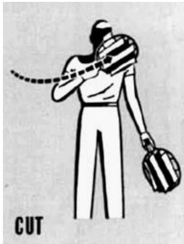
Then the LSO's paddles flashed quickly into the classic 'cut' signal. The pilot instantly responded, cutting his throttle. Later, as Swede Vejtasa recalled: "At that instant, I was looking right at the ramp."
