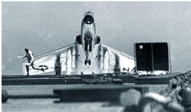
By the mid-1950s, American aircraft carriers were being built with angled flight decks and outfitted with optical landing systems [example depicted on the right]. Initially, it was thought this invention would allow a pilot to land without help from a LSO. However, accident rates actually increased when the human factor was removed from the equation.
