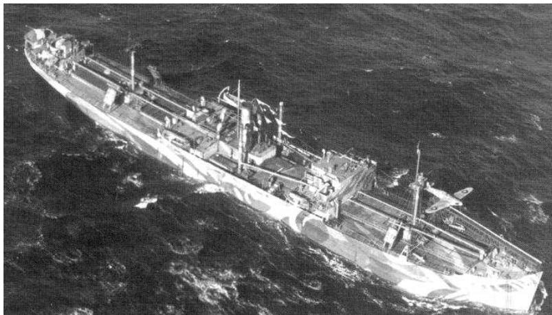
**Catapults & Aircraft:** The catapults were complex devices perched precariously high on a ship's bow, as this image indicates. Nevertheless, there is no record of any failures of a catapult under combat conditions. In addition to an RAF pilot, each catapult equipped vessel carried a cadre of aircraft and catapult maintenance personnel.
