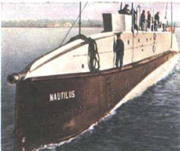
These included a cushioning bowsprit 12 feet long to act as a bumper, an ice drill to provide access to the surface in case the submarine was unable to break through the ice, a telescoping escape trunk, an emergency air intake system, and a diving chamber. Her conning tower and periscope were modified to be retractable. The most obvious change was the addition of a large wooden superstructure placed atop the sub's hull.
