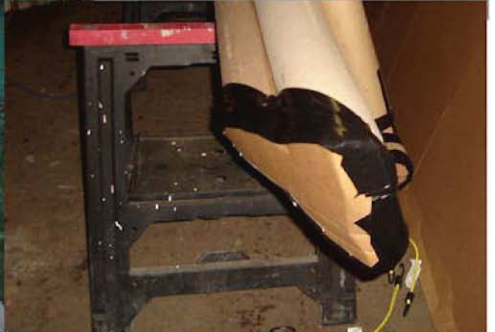
Cardboard Straps to hold Frame to Hull
